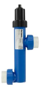
The UV-C radiation inactivates bacteria, viruses and other microorganisms and stops them from multiplying. This can reduce your chlorine concentration up to 50%! Max. pressure: 1 bar. 50mm connections included.
